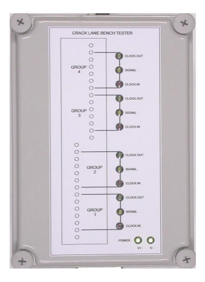
Tester accepts older Crack Lanes ( cables that plug into the bottom ) and the newer Sealed Crack Lanes ( cables sealed into the bottom ).
